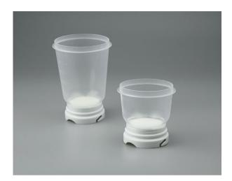
An all-in-one sterile and ready-to-use filter consists of a funnel, a gridded membrane and a base support in one unit. Click-fit closure, easy to use. From taking the sample until incubation in just a few easy steps, minimizing the risk of secondary contamination. They have been specifically designed for the detection of microorganisms in pharmaceuticals, food, beverages, water and other liquids.
