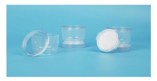
The all-in-one sterile and ready-to-use filter units consist of a funnel, a white gridded MCE membrane with a petri dish. After the sample is filtered, remove the upper funnel and the base can convert into a petri dish. Every filter unit is individually packaged and ready for use. It is easy to operate and minimizes the risk of secondary contamination.
