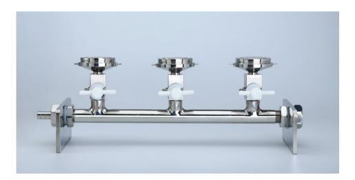
The manifold is made of 100% high quality stainless steel that is easy to sterilize and clean. There is no need for disassembly, just place the manifold into the autoclave device and set the temperature at 121°C for 30 minutes for sterilization. To secure the filter adapters, simply push them into the manifold and choose your preferred positions from the 3 or 5 available working positions.
